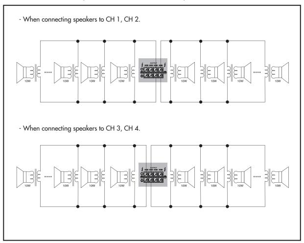
\* Caution: 1. Make sure that the total impedance does not equal or less than the rated impedance.
